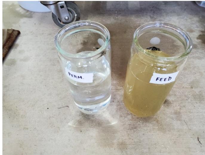
Produced Water treatment-Raw water 132 NTU Permeate <0.5 NTU- Permian Basin New Mexico
