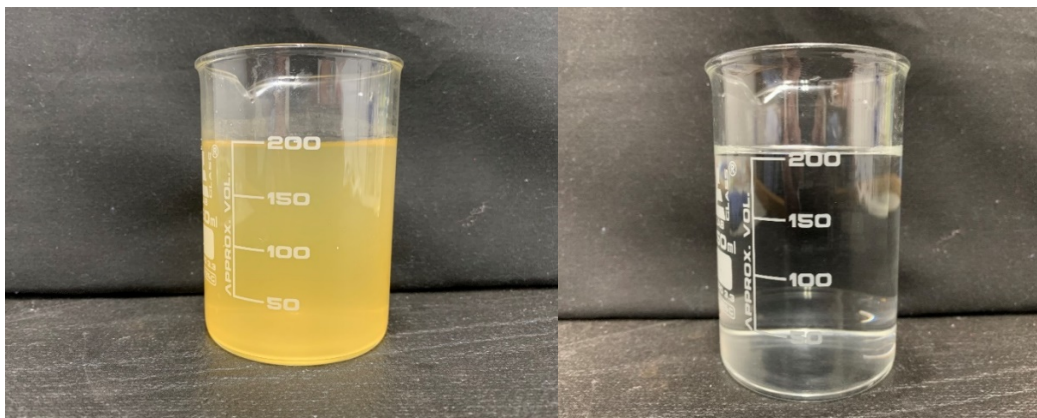
Produced Water Treatment Raw water 161 NTU Permeate <0.3 NTU- Permian Basin Texas
