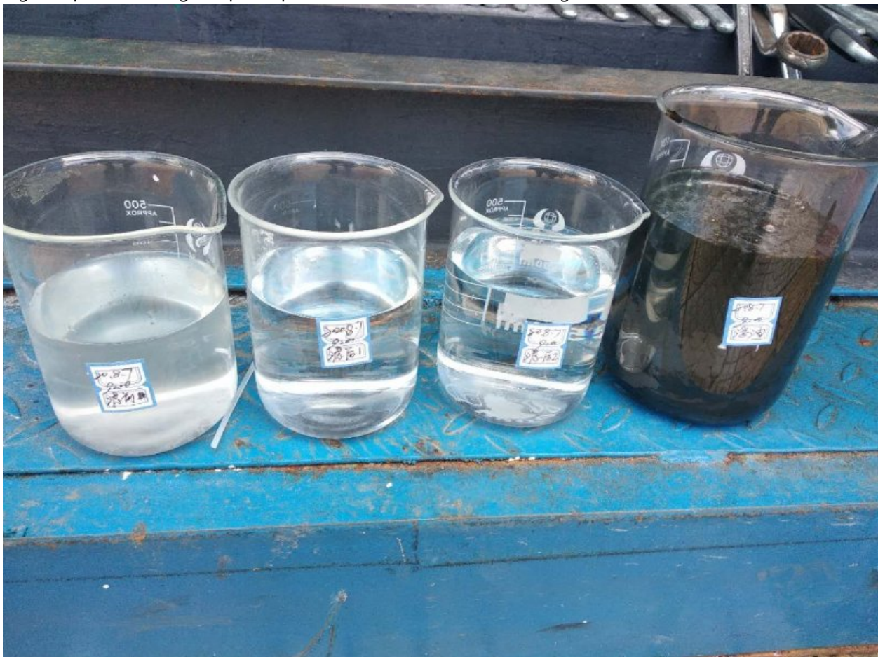
Left -Raw produced water: Center-Permeate- housing 1 and 2; Quality-1 ppm oil, <1ppm TSS,<1 micron: Right – Oil separated in Housing and automatically drained from housing
