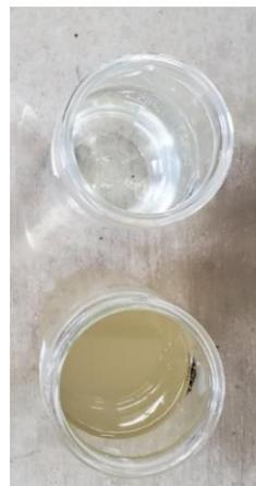
The **RSL Membranes™** were applied to the same water using a small 3 bbl/day test unit and consistently reduced turbidity from 130 NTU to less than 0.4 NTU.
