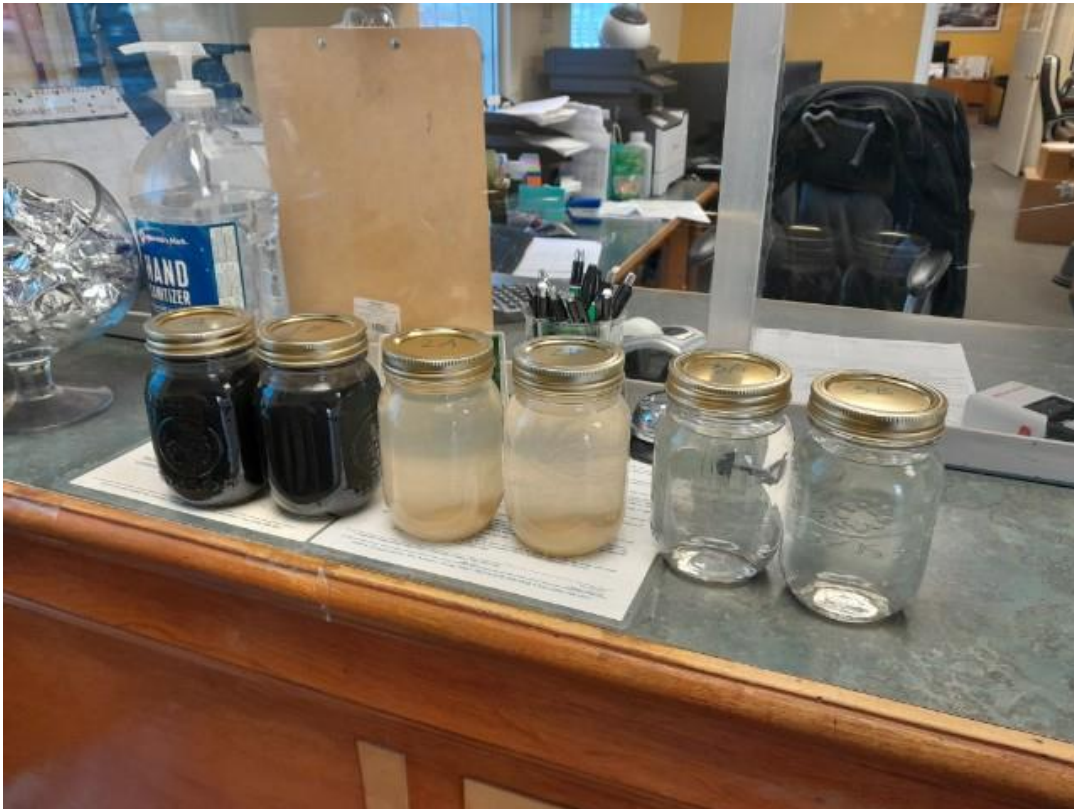
Figure 26: Duplicate samples of Raw water without H 2 O 2 , Raw water with H 2 O 2 , and RSL Membrane treated water(permeate).
