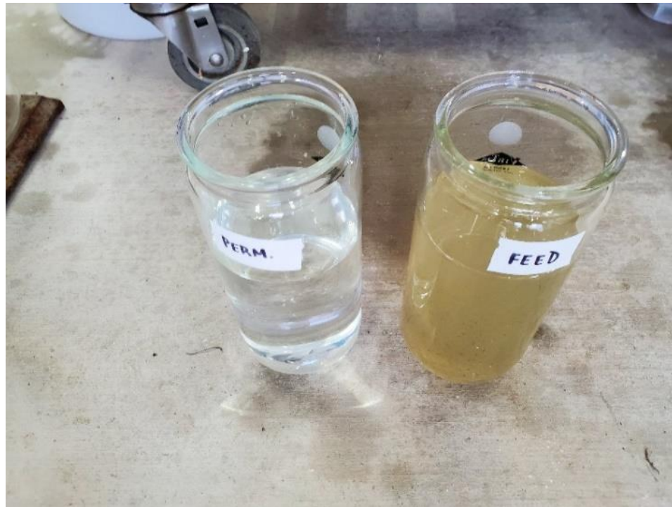
Figure 12: Feed water and Permeate from 25 m 3 /hr replaceable skin layer membrane— Petro China-Dajing Production Zone
