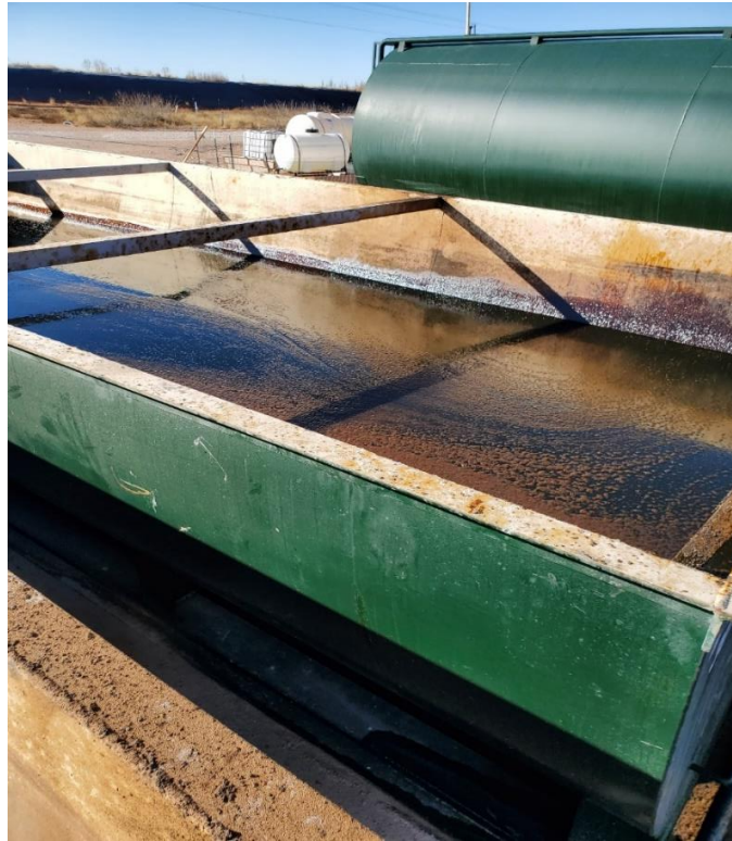
Figure 19: Frack tank containing Backwash (Water, Oil and Solids) resulting from Produced Water Treatment using Replaceable skin layer membranes
