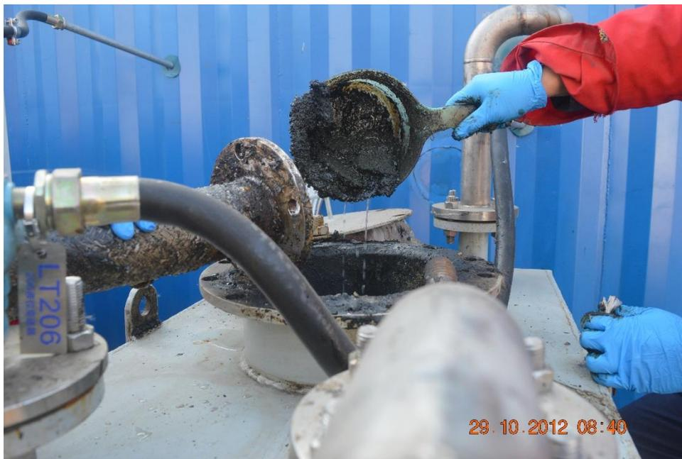
Figure 2 shows the collection of oil that is separated in the housing. In this case the oil is a heavy oil and the system was operated at 70<sup>o</sup> C to allow a lower viscosity oil to be separated. The concentration of oil can impair the solids separation however a method has been
