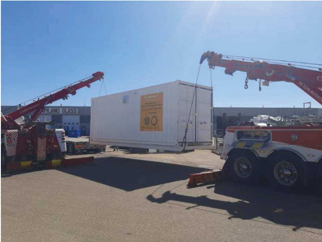
Figure 24: Easy Mobility for the replaceable skin layer membrane Treatment Unit 100 m 3 / hr being moved from Barstow, Texas to a southern Texas E & P Operator Site.
