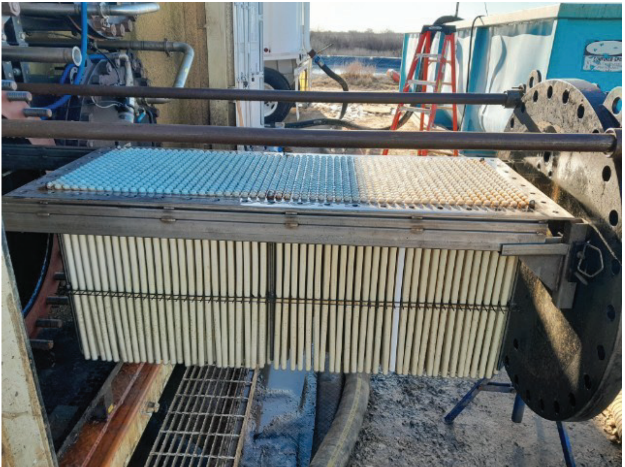
Figure 25 The Replaceable skin layer membranes after two months of operation with the slide out tray for easy maintenance.
