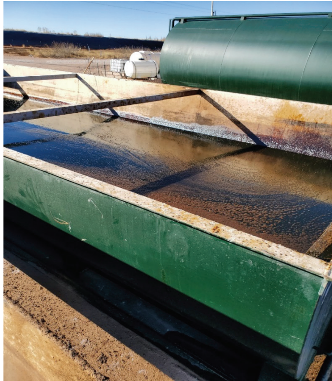
Figure 19: Frack tank containing Backwash (Water, Oil and Solids) resulting from Produced Water Treatment using RSL Membranes™
