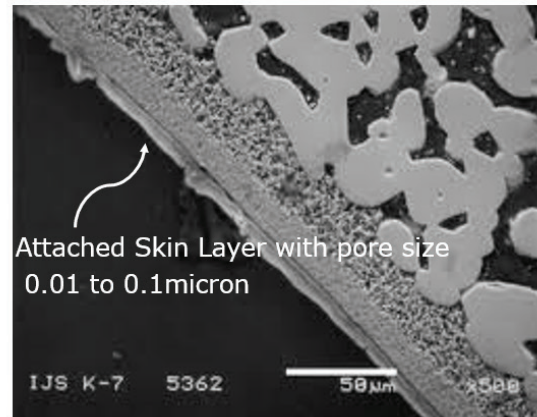
Generation 2 - Fabricated and attached skin layer membranes-Most common
