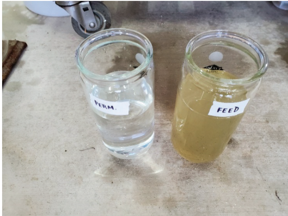
Figure 9: Feed water and permeate from 25 m 3 /hr replaceable skin layer membrane— Petro China-Dajing Production Zone
