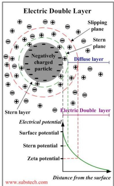
The right side of figure 1 shows the electric potential decreasing over distance from the surface. The electric potential defines the intensity and width of the EDL.
