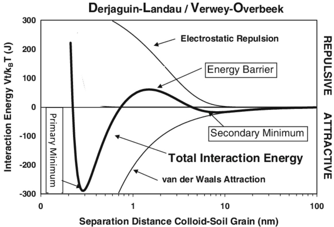
Figure 5 – Sum of Van der waal and EDL Forces = Energy or Force Barrier
