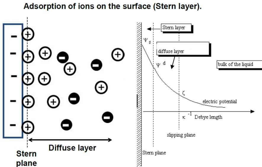
Figure 1: The Stern and Diffuse layer of the Electric Double Layer (EDL) showing a force of repulsion that diminishes over distance from the surface of the colloid
