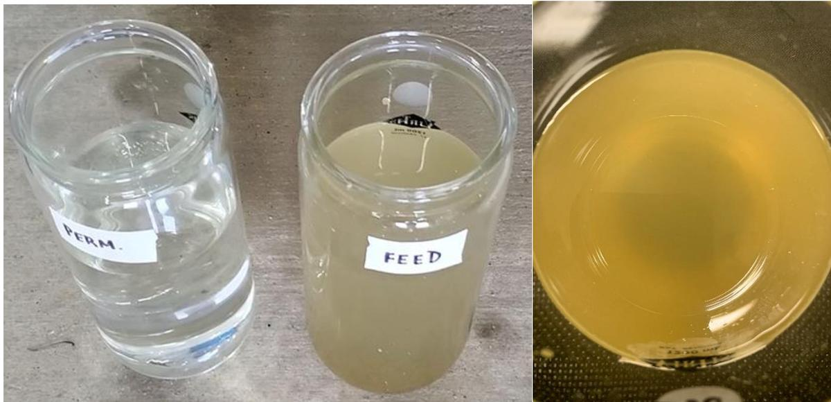
Figure 7: (Left) Permeate from **RSL Membrane™**, (Center) Feed water, (Right) Top View of Feed
