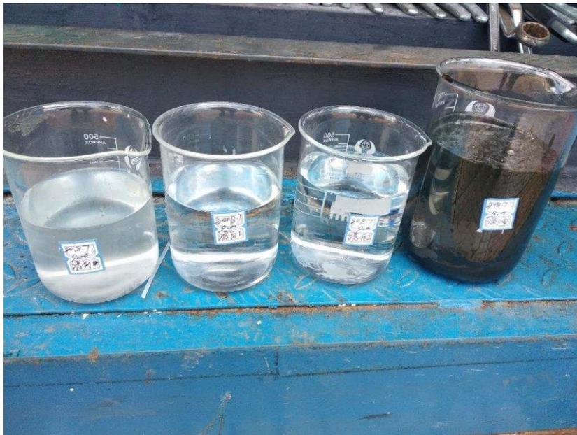
Left -Raw produced water: Center-Permeate- housing 1 and 2; Quality-1 ppm oil, <1ppm TSS,<1 micron:
