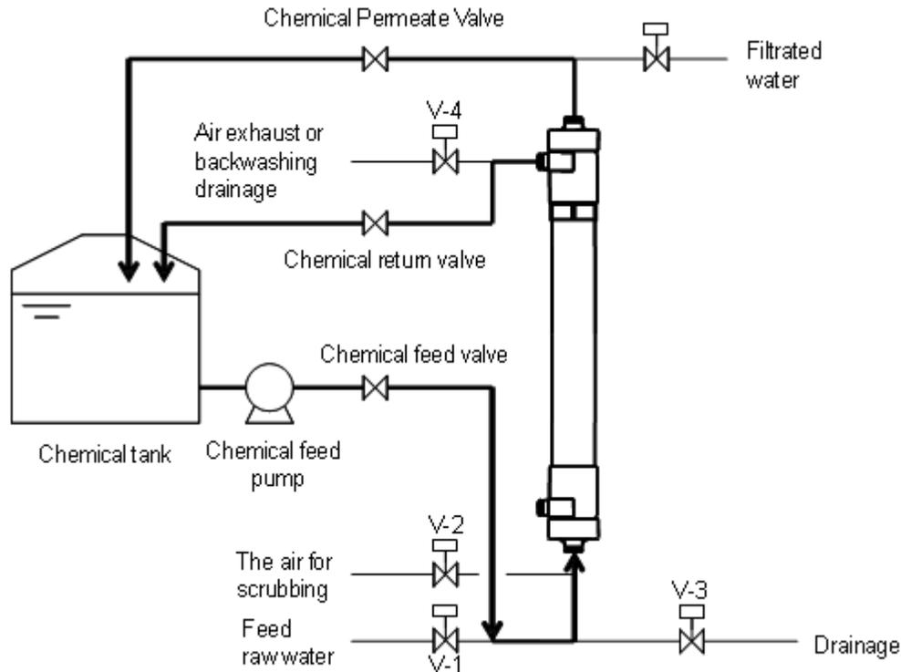
Figure 3: Clean-In-Place (CIP) Schematic
