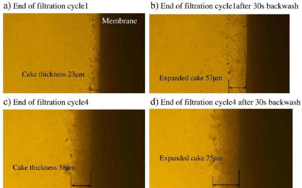
Figure 2 – Fouling cake at the end of filtration cycles, and after 30s backwash without air scouring. Filtration flux 50 l/m<sup>2</sup>-h, filtration duration 3570s, backwash flux 50 l/m<sup>2</sup>-h, backwash duration 30s. Feed solution: 50 mg/L bentonite and 50 mg/L alginate. (Ye et al., 2011)
